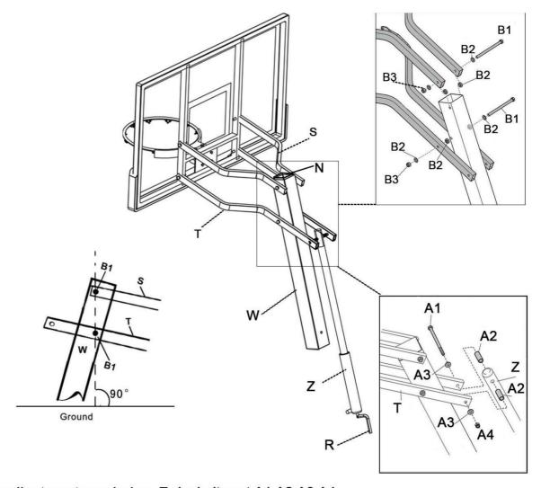
Install adjustment machnism Z, by bolts set A1,A2,A3,A4.
