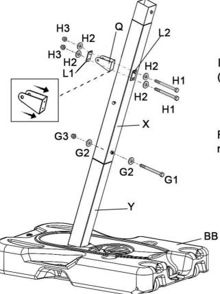
Install 2pcs main poles X, Y together (by bolts set G1,G2,G3).
