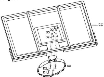
Install the backboard brace S, T on the back of backboard CC as shown.
