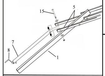
9 Finally, install whole assembled basketball system to the bottom main pole by bolt(18). tighten all the nuts on bolts.
